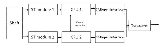
For safety-related applications this encoders shall be used in combination with a safety-related master (PLC). This PLC shall compare the position values of both channels to each other and on deviations greater than 1 % of the measuring range the PLC shall transit the machine into inherent safe state.
