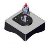
Step 2: Place spacer tool around shaft. Slip hubdisk assembly onto shaft and slide down until it bottoms out against spacer tool. Note: Alternate spacer orientations may be required depending on the base/mounting configuration
