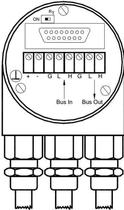
**Fig. 1 Connection cap bus in and bus out**
