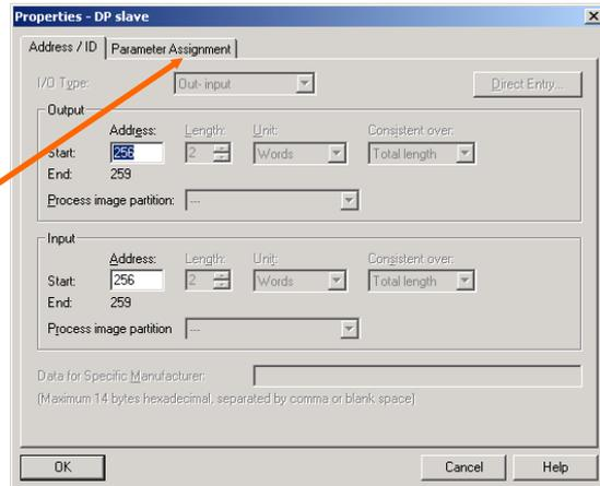
After choosing the „Device-specific parameters“ the different parameters (depend on the encoder version) can be set.
