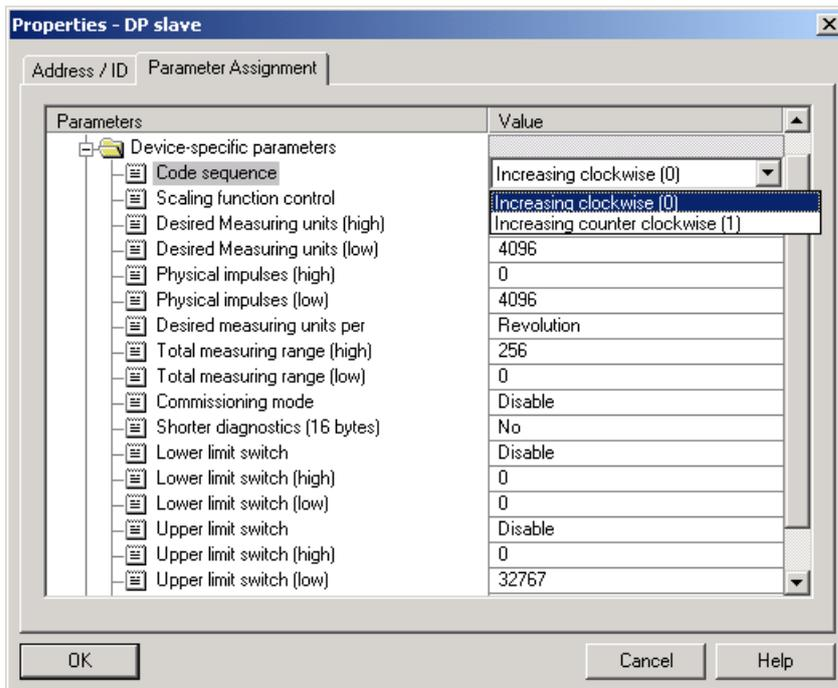
Due to the old versions of software tool STEP7 32-bit parameter values (e.g. total measuring range, software limit switches) have to be divided into high and low word. This is not necessary with the new STEP7 versions and our actual GSD file.
