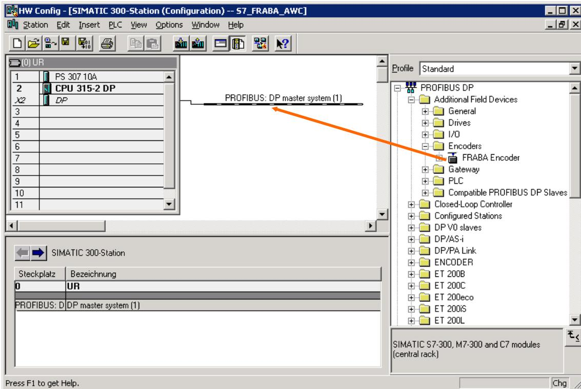
After inserting the Profibus master system in the hardware configuration (“Insert” – “Master System”) the FRABA encoder can be chosen from the hardware catalogue and added to the Profibus network: Select the device “FRABA Encoder” and drag it with the mouse to the network (or choose the network and double click the “FRABA encoder”). Now the slave address has to be entered (has to be equal to the address setting in the connection cap).
