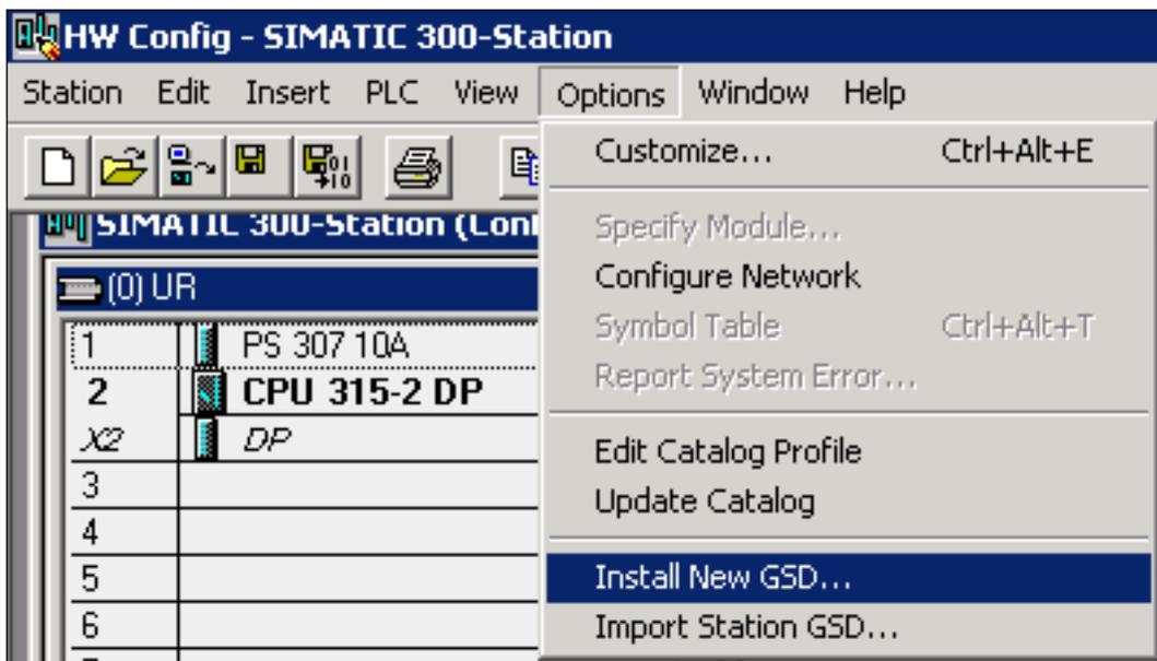
After the successful installation of the GSD file the FRABA encoder can be found in the hardware catalogue under „PROFIBUS-DP“ – „Additional Field Devices“ – „Encoders“ – „FRABA Encoder“.
