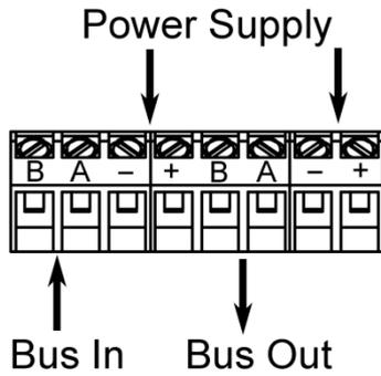
The power supply has to be connected once (no matter which clamps). If the terminating resistor is switched on, the outgoing bus lines are disconnected.
