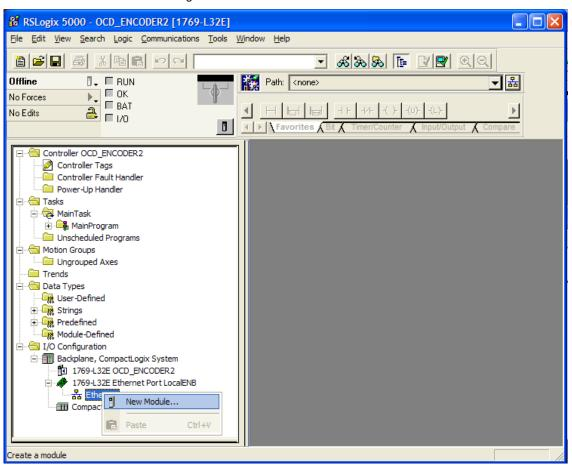
To use a Generic Device select the Generic Ethernet Module. Some PLC's support Encoder Devices too. Please check that the matching EDS file complies with the configuration of the encoder. The device type is programmable.
