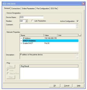
The cycle time (RPI), the input and output configuration can eb checked in tab *Connections* under *General*. The offline parameters are available Under *Configuration*
