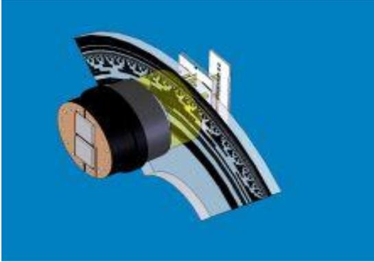
The measuring system in the single-turn module consists of a light source, a code disc pivoted in a precision ball bearing and an opto-electronic scanning device. A LED is used as a light source which shines through the code disc and onto the screen behind. The tracks on the code disc are
