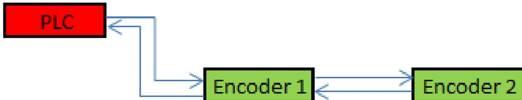
The line structure can be built up like known from standard field bus systems e.g. CANopen. The sensor can be connected to other devices by usage of “straight” or crossover network cable, because the PHY of the encoder is capable to realize Auto crossover. You need at least a cable of category Cat5e to get a data transfer rate up to 100 Mbit. To increase noise immunity only cables with foil and copper netting shield should be used (S/UTP), twisted pair, AWG26.
