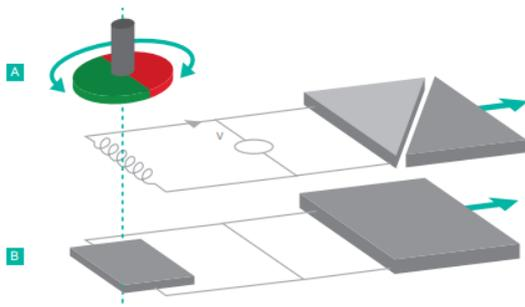
POSITAL can also provide absolute multiturn measurements by means of a revolution counter system that uses an energy harvesting system based on the Wiegand effect. This system requires no gears or batteries. Eliminating batteries brings about many advantages. Batteries have a limited lifespan, weigh a lot, and often contain harmful
