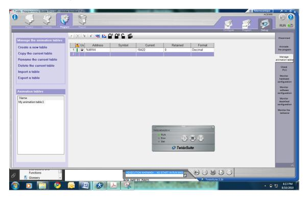
The position Readout is 18416 through the memory location %MW4 (Shown in the programming). We know that the resolution is set to  $0.01^{\circ}$ . TILTIX Position Value =  $18416 \times 0.01^{\circ} = 184.16^{\circ}$
