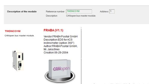
Once the TILTIX EDS file is being uploaded all objects – including the PDOs – are added to the controller. The Schneider system automatically
