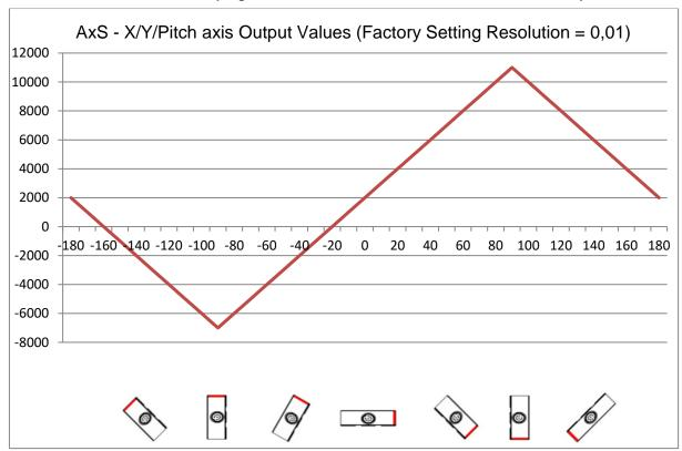
Explanation: The position limits are adjusted to  $\pm -90^\circ$  + offset. When an offset of  $\pm 20^\circ$  is programmed, the overall output range will be adjusted to  $\pm -70^\circ$  to  $\pm 110^\circ$  as seen in the graph. The result is that the turning point where the graph switches from positive to negative slope stay at the physical position of  $\pm -90^\circ$ .
