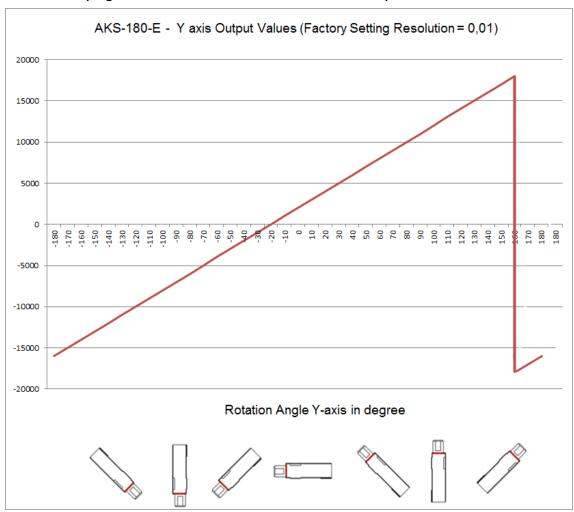
Explanation: The position limits stay +/- 180°. This results that the jump from 180° to -180° will be shifted according to the programmed preset, as seen on the graph.
